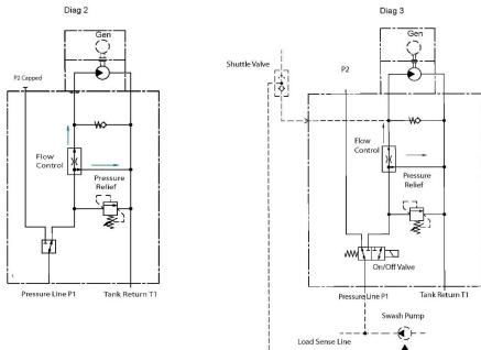
Diagram 1. Illustrates connection onto a fixed displacement pump with other functions required, Diagram 2. Is a simple on/off system from a fixed displacement pump and Diagram 3. Is for variable displacement pump.
